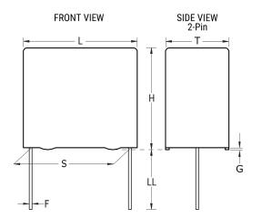
**General Information** Series F461 Dielectric Metallized Polypropylene Style Radial MKP, Pulse Features RoHS Yes Lead Cut/Short AEC-Q200 No Component 4.34 g Weight The Rated Voltage Decreases 2%/C Between +85C And +105C (1.25%/C For AC). ClimCat: Miscellaneous 55/105/56.
