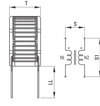
General InformationSeriesSCFStyleThrough-HoleRoHSYesNotesLead Spacing (S/S1) Are For Reference Only.MiscellaneousTemperature Rise Maximum: 50 KCoreNanocrystal
