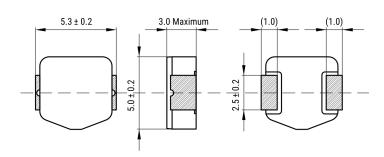
Series MPX Style SMD Chip Size 0530(2120) Description Surface Mount Inductor Features Power Inductors **RoHS** Yes Core Composite Miscellaneous 40 (K) Temperature Rise Max.
