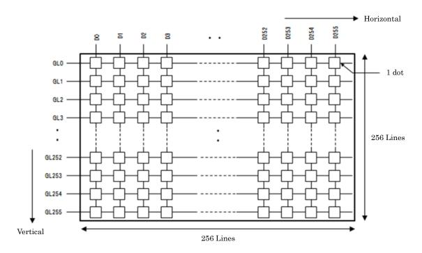
Addressing of Gate line (GL\*) to be selected is necessary for vertical direction. Rewriting data for one line is necessary for horizontal direction due to rewriting one line at once.
