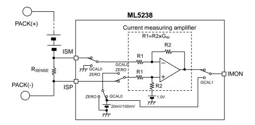
If the current is zero,  $V_{IMON}$  = 1.0V, in the discharging state,  $V_{IMON}$  > 1.0V, in the charging state,  $V_{IMON}$  < 1.0V.
