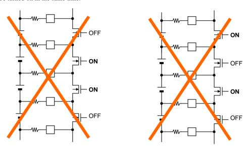
IC heats by cell balancing current and cell balancing switch resistor, restrict the number of switches of ON and time of ON, in order to keep the power consumption of cell balancing switch less than allowable power dissipation,
