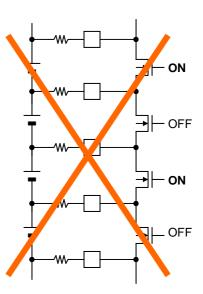
IC heats by cell balancing current and cell balancing switch resistor, restrict the number of switches of ON and time of ON, in order to keep the power consumption of cell balancing switch less than allowable power dissipation,
