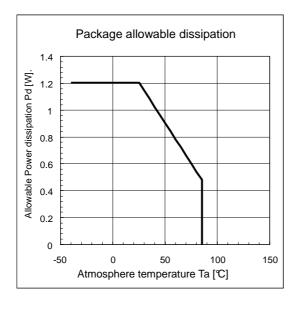
Package loss tolerant decreases as the atmosphere temperature (Ta) increase. If VREG pin output load current is large, make the power loss smaller than the value shown in this figure.
