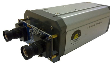
TI/Leopard Imaging Dual Image Sensor Camera
