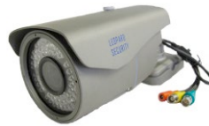
TI/Leopard Imaging HD-SDI camera utilizing LatticeECP3
