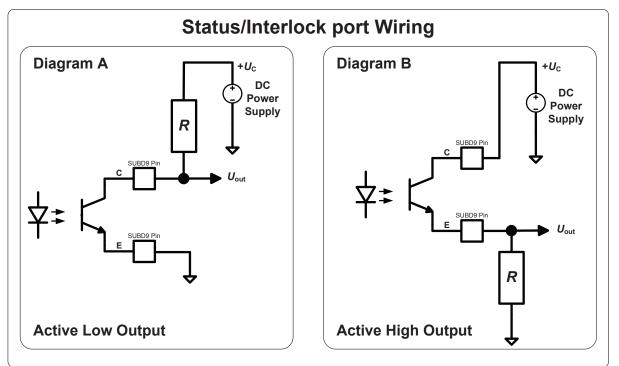
In the Diagram A Active Low Output, the output signal  $U_{out}$  switches to GND when the corresponding LED is ON. In the Diagram B Active High Output, the output signal  $U_{out}$  switches to  $+U_c$  when the corresponding LED is ON. When the output signal  $U_{out}$  is switched to GND, its value is lower than 0.2 V. When the output signal  $U_{out}$  is switched to  $+U_c$ , its value is equal to  $+U_c$ .
