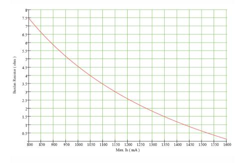
To maintain safe start-up  $R_{\rm M}$  must not exceed 3  $\Omega$  during fault condition.
