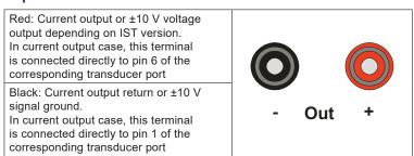
Two "Banana" jacks, located on the back panel of the IST ULTRASTAB, allow the connection of the secondary current outputs or the ±10 V voltage outputs to the measurement device.
