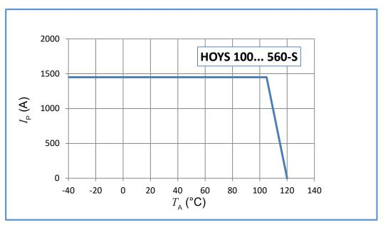
Important notice: whatever the usage and/or application, the transducer primary bar / jumper temperature shall not go above the maximum rating of 120 °C as stated in page 3 of this datasheet.
