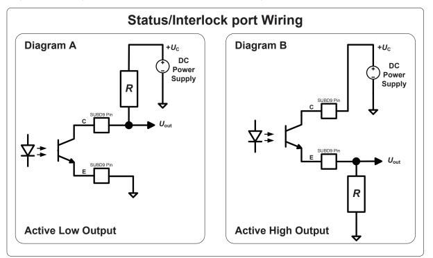
In the Diagram A Active Low Output, the output signal  $U_{out}$  switches to GND when the corresponding LED is ON. In the Diagram B Active High Output, the output signal  $U_{out}$  switches to  $+U_c$  when the corresponding LED is ON. When the output signal  $U_{out}$  is switched to GND, its value is lower than 0.2 V. When the output signal  $U_{out}$  is switched to  $+U_c$ , its value is equal to  $+U_c$ .
