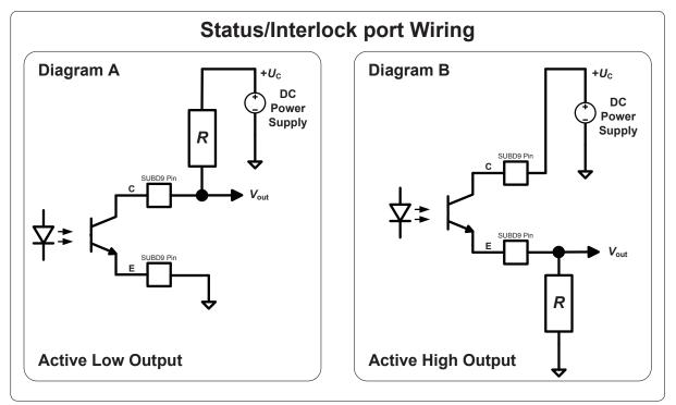
In the Diagram A Active Low Output, the output signal  $V_{out}$  switches to GND when the corresponding LED is ON. In the Diagram B Active High Output, the output signal  $V_{out}$  switches to  $+U_c$  when the corresponding LED is ON. When the output signal  $V_{out}$  is switched to GND, its value is lower than 0.2 V. When the output signal  $V_{out}$  is switched to  $+U_c$ , its value is equal to  $+U_c$ .
