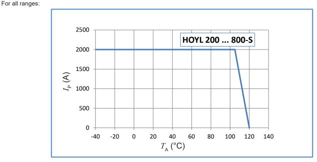
Important notice: whatever the usage and/or application, the transducer primary bar / jumper temperature shall not go above the maximum rating of 120 °C as stated in page 3 of this datasheet.
