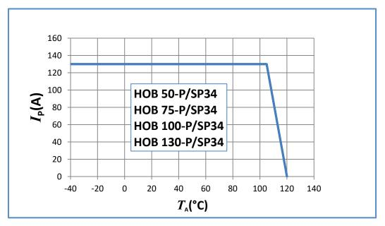
Important notice: whatever the usage and/or application, the transducer jumper temperature shall not go above the maximum rating of 120 °C as stated in page 3 of this datasheet.
