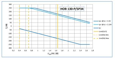
$U_{\rm ref}$  (IN) Min-Max defines the recommended interval in order to reach the  $I_{\rm P\ max}$  range (asymetrical and positive value only).
