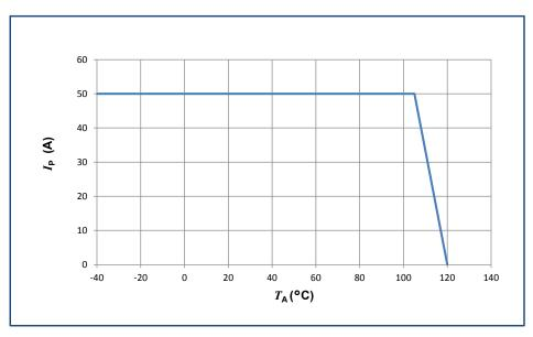
Important notice: whatever the usage and/or application, the transducer primary bar / jumper temperature shall not go above the maximum rating of 120 °C as stated in page 2 of this datasheet.
