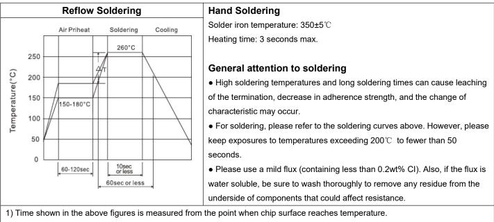
2) Temperature difference in high temperature part should be within 110°C.
