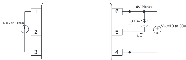
Figure 16 : I_{OH} Test Circuit
