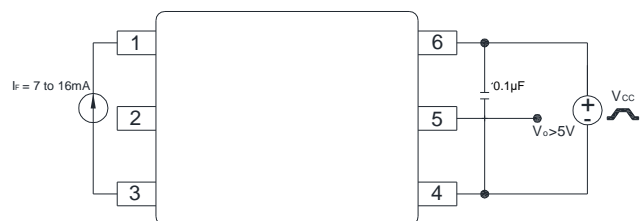
Figure 19 : U_{VLO} Test Circuit
