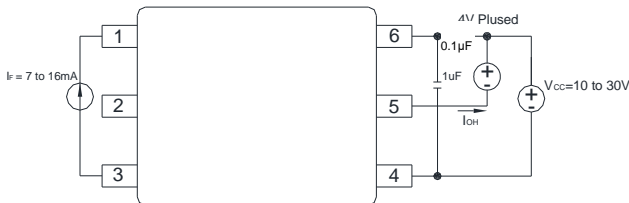
Figure 16 : I OH Test Circuit
