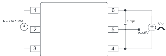
Figure 19 : U VLO Test Circuit
