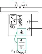
V = Voltage C = Common, Transfer Contact NO = Normally Open NC = Normally Closed
