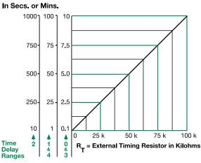
This chart applies to externally adjustable part numbers. The time delay is adjustable over the time delay range selected by varying the resistance across the RT terminals; as the resistance increases the time delay increases. When selecting an external RT, add the tolerances of the timer and the RT
