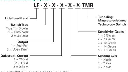
Example: LF21215TMR is an Omnipolar, PushPull, 1.5uA, X axis, 17 Gauss Note: Every combination is NOT offered. Contact Littelfuse for availability.
