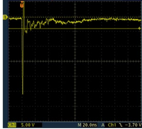
SP1124 IEC 61000 -4-2 -8 kV Contact ESD Clamping Voltage
