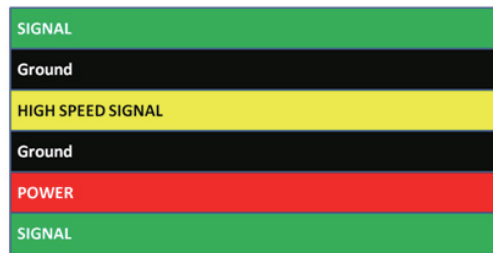
Figure 2: Typical multilayer PCB stack up, best to route data between ground planes to eliminate radiated noise and improve Signal Integrity.
