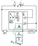
V = Voltage C = Common, Transfer Contact NC = Normally Closed NO = Normally Open S1 = Initiate Switch UTL = Untimed Load
