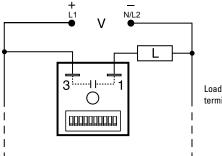
Load may be connected to terminal 3 or 1.
