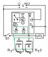
V = Voltage C = Common, Transfer Contact NC = Normally Closed NO = Normally Open S1 = Initiate Switch UTL = Untimed Load
