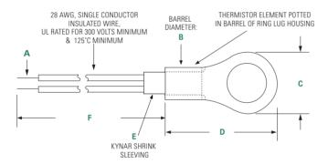
Dim "L" is the MIN lead wire length, and is specified by the last two digits of the part number (USUR1000-xxx-xx) e.g. USUR1000-102G-03 would have a MIN lead wire length of 3"
