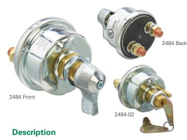
2484 Series Battery Disconnect Switches are 36V Single Pole, Single Throw (SPST) manual disconnect switches that can be used to disconnect the battery from the vehicle electrical system. Disconnecting the battery from the electrical system prevents potential thermal events and ensures system shut down during maintenance or emergency. Battery disconnect switches also prevent parasitic loads from draining the battery during inactivity.
