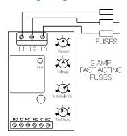
L1, L2, L3 = Line Voltage Input NO = Normally Open Contact NC = Normally Closed Contact C = Common, Transfer Contact
