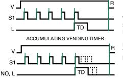
V = Voltage S1 = Initiate Switch NO = Normally **Open Contact** L = LoadTD = Time Delay R = Reset
