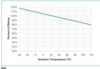
Rerating depicted in this curve is in addition to the standard derating of 25% for continuous operation.
