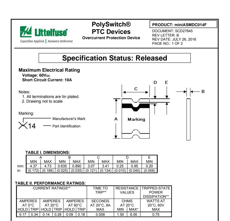
\* Maximum resistance is measured 1 hour after reflow.
