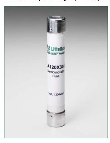
Littelfuse LA120X semiconductor protection fuses, rated ½ through 30A, 1200 VAC are popular for use in traction drive auxiliary circuits and similar applications. LA120X fuses are also suitable for use on 1000VDC auxiliary circuits with low time constants.
