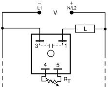
Load may be connected to terminal 3 or 1.  $R_{\tau}$  is used when external adjustment is ordered.
