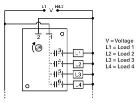
SC4 shown. For SC3, terminal 6 and load L4 are eliminated.
