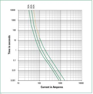
For 50 A rating, it may not break current consistently when overload current is less than 200%  $\ln$  (represented by dotted portion of this Time Current Curve), as may be arc current continuously pass through fuse under this condition. Do not recommend to use conditions of below 200% In overload.
