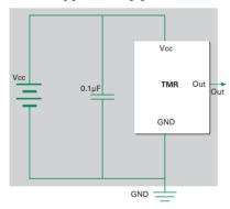
Note: It is strongly recommended that an external bypass capacitor be connected in-close-proximity to the device between the supply and ground pins to reduce noise. The recommended value for the external bypass capacitor is 0.1µF.
