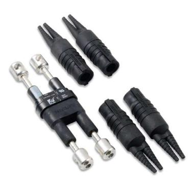
LEXT-YY-S and LEX-YYC-S series breakaway fuseholders meet state and federal highway commission safety standards requiring fuseholders to readily disconnect from power in case of a pole knockdown. The breakaway feature consists of a receptacle permanently attached to the power line and a fuseholder with matching terminals. If a knockdown occurs, the parts separate leaving the energized conductor recessed and unexposed.
