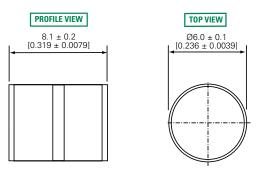
'R' Type Radial Lead Devices (SL1003AxxxR and SL1003AxxxRF)
