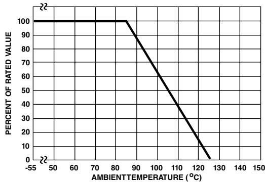
Figure 1A - Power Derating for Epoxy Coated
