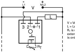
V = Voltage L = LoadR<sub>T</sub> is used when external adjustment is ordered.
