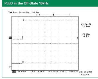
Channel 1: current through LEDs (318 mA) Channel 2: voltage across PLED device (4.5 V)
