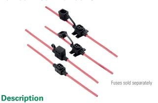
The FHC In-Line Fuse Holder is the perfect solution for applications requiring the circuit protection of a JCASE® Fuse (20A - 60A) but have the space constraints requiring a low profile option. The FHJ In-Line Fuse Holder paired with a JCASE Fuse offers size and weight savings compared to MAXI® fuse holders, and has an optional protective cover for splash resistance or a mounting bracket.
