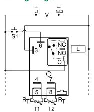
NO = Normally Open S1 = Reset Switch C = Common, Transfer Contact L = Load
