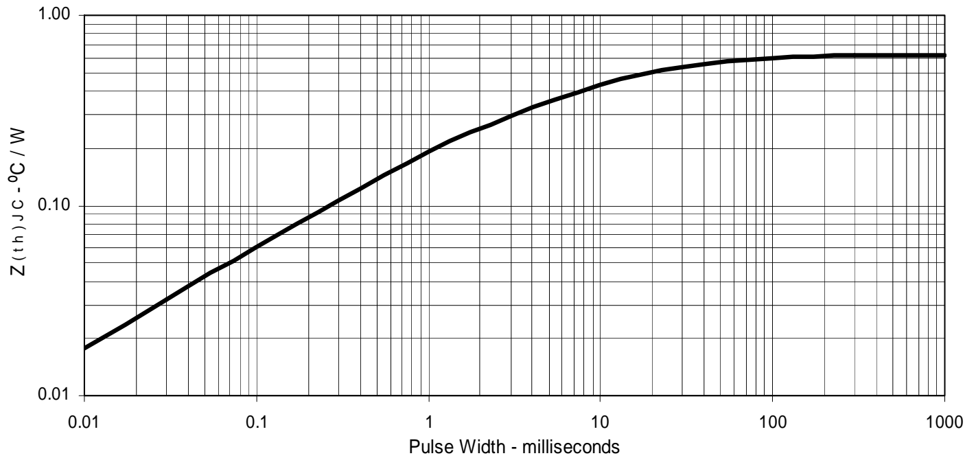
Fig. 13. Maximum Transient Thermal Impedance
