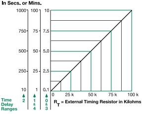
This chart applies to externally adjustable part numbers. The time delay is adjustable over the time delay range selected by varying the resistance across the RT terminals; as the resistance increases the time delav increases
