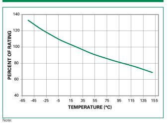
Re-rating depicted in this curve is in addition to the standard re-rating of 20% for continuous operation.
