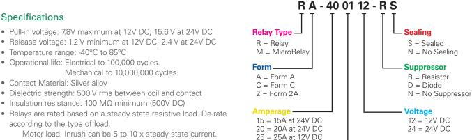
Solenoid load: Inrush can be 10 to 20 x steady state current. Incandescent lamp load: Inrush can be 10 to 15 x steady
