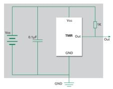
Note: It is strongly recommended that an external bypass capacitor be connected in-close-proximity to the device between the supply and ground pins to reduce noise. The recommended value for the external bypass capacitor is  $0.1 \mu F$ .
