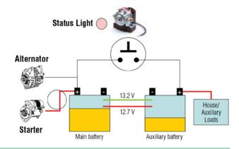
The engine is powering the alternator, and the starting battery has reached 13.2V. Only now does the Smart Battery Isolator reconnect, enabling the depleted auxiliary battery to be charged. By not reconnecting until the main battery is charged, the alternator is protected from excessive loads. 6 Now both batteries are charged again.
