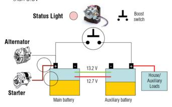
**2** The boost switch is pressed. It closes the Smart Battery Isolator solenoid for one minute. Now the power in the auxiliary battery is available for starting.
