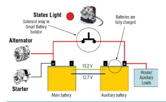
2 When the engine is turned off, the alternator no longer supplies a charge to the batteries, and the loads on the batteries begin to deplete them.
